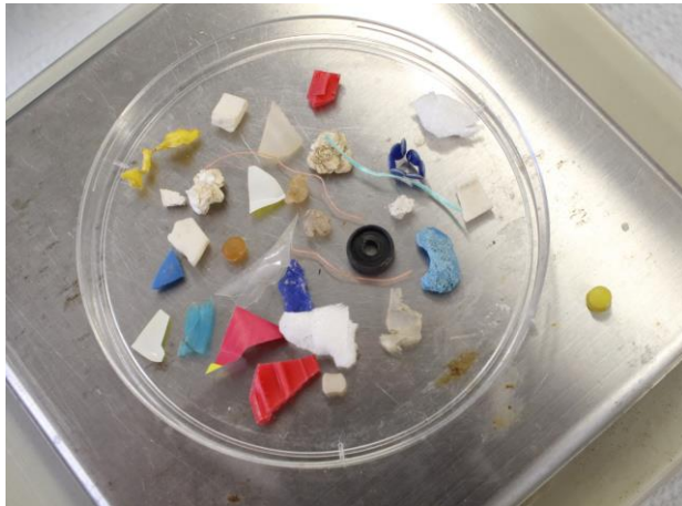
Fulmar stomach contents sample. Approx. 0.35 g of plastic pieces. The yellow industrial granule on lower right of image is provided for scale and is 3-4 mm in diameter. The actual sample is contained within the circular petri dish which is resting on a digital balance. This was one of the samples made in the Dove Marine Laboratory on 26 Oct 2017.
