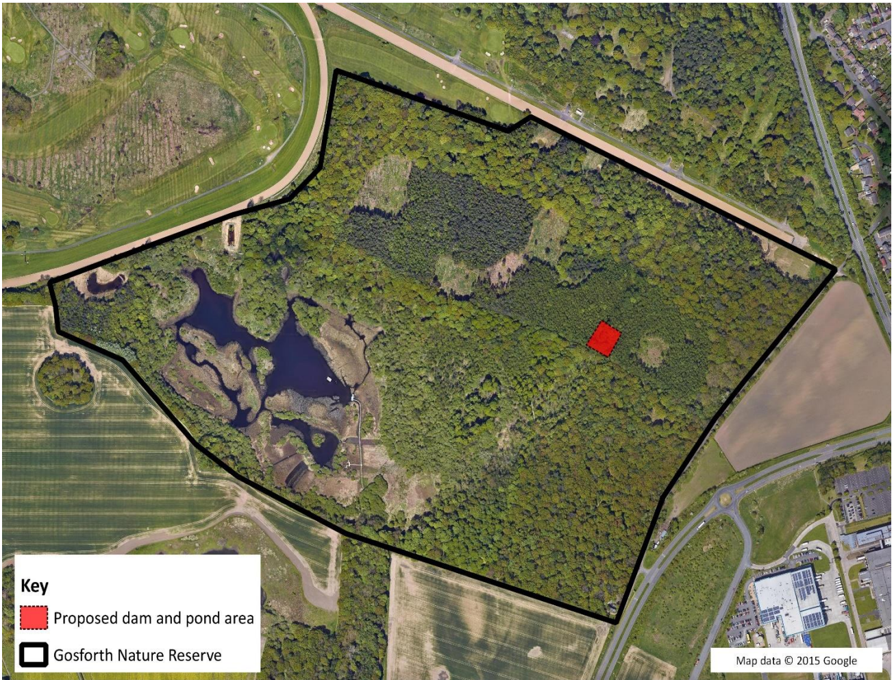
Map 6. Proposed area for felling of regenerated Birch to create an inundation pond and install a gabion dam across the Whitecroft Burn.
