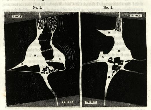
The above are two sections, or profiles, of one of the Riders (marked a on the plan), as shewn on the two sides of the working that had crossed it, and which was about four yards wide.
