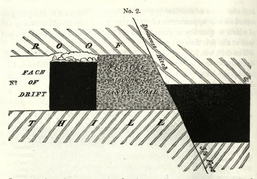
It was evident that a quantity of inflammable air had been contained in this cavity, in a high state of compressure, and that on the Coal being worked away, till it was no longer equal to resist the elastic force of the compressed gas, the gas had escaped, with a sort of explosion, displacing the block of Coal, filled the adjoining workings, and fired at the first lights it met with, after being brought down to the firing point by a due admixture of atmospherical air.
