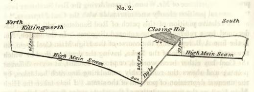
Killingworth House which is, as before stated, about 950 yards north of the Dyke, is built upon the Grindstone Post, a well-known Sandstone bed here at the surface; but, if we wished to find that bed at the Dyke, we should have to sink 120 fathoms before we reached it.
