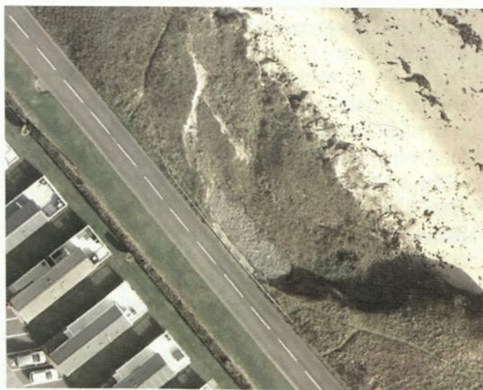
Figure 7. Landslip in superficial (drift) geological deposits at Cresswell in Northumberland.
